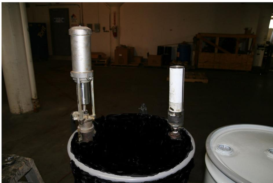
After mixing, replace lid and seal tightly. Use collars on drum pumps and use moisture desiccants on the isocyanate (Component "A") drum.
