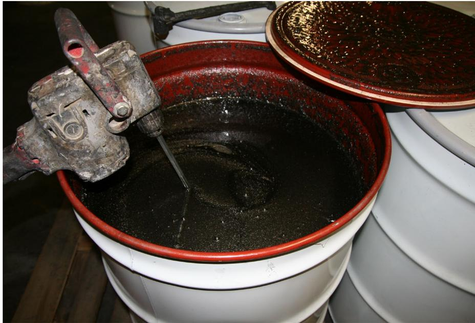
When mixing, ensure blade touches bottom of drum to mix any particles that may have settled to the bottom during shipping/storage. Mix thoroughly from side-to-side and from top-to-bottom. After mixing is complete, replace lid and tighten ring.
