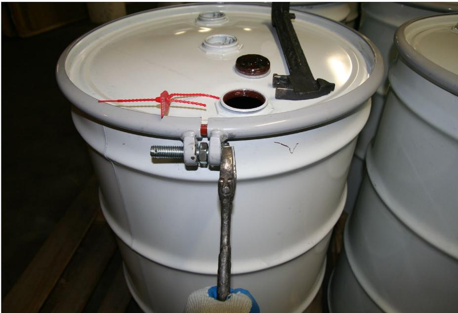
**Remove red drum tag/seal and loosen bolt. Do not remove until all pressure in container has been relieved.**
