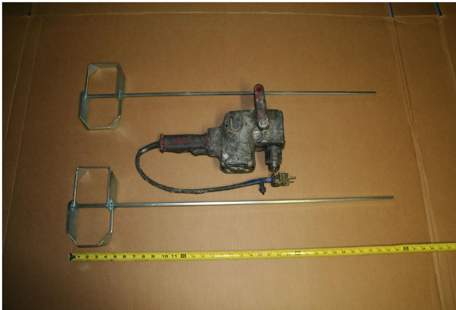
Electric drill with drum-length mixing blades. Separate blades are needed for each component.
